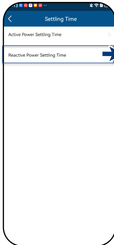
Fig. 162. Select reactive power settling
