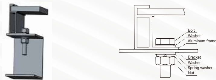
Figure 5 Bolt Installation of Mono-facial Modules
